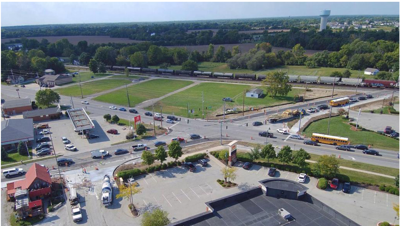
Right turn lanes made at the intersection of CR 600W and Broadway have helped provide a smoother flow of traffic.
